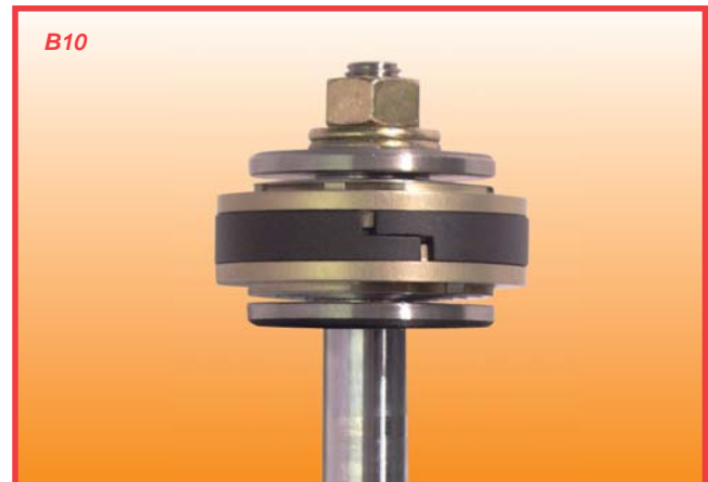
Place piston washer & nut on piston rod
