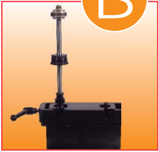
B1 Clamp the head assembly into the vice
