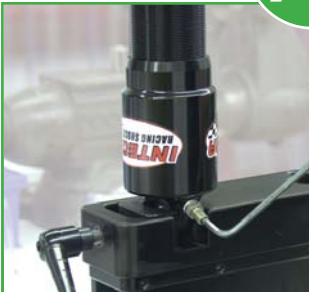
A1 Discharge nitrogen gas prior to disassembly
